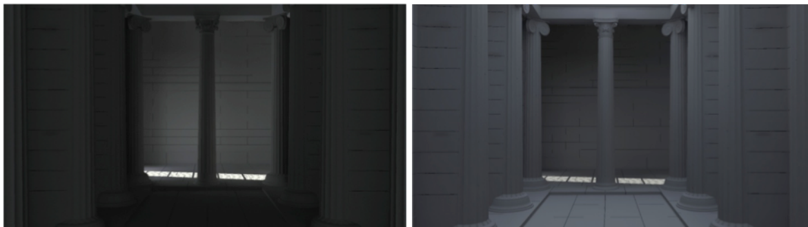
Figure 25. Comparison of the interior's illumination between the closed roof (left) and hypaethral roof at dawn of spring equinox.
